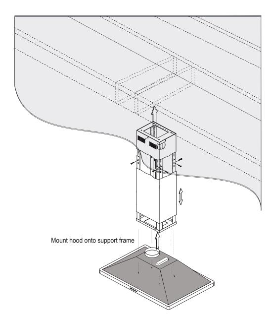
6. Lift lower duct cover and hood body onto bottom of support frame.
